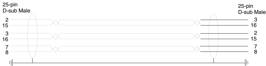
Cable between two terminals for RS-422 communication
